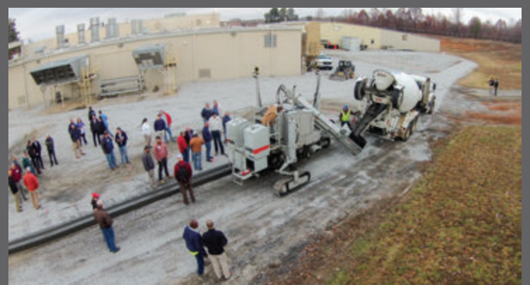
Far left – Power Curbers' Product Support team and representatives from Topcon put on demonstration pours using a flyash mix with the 5700-C.
