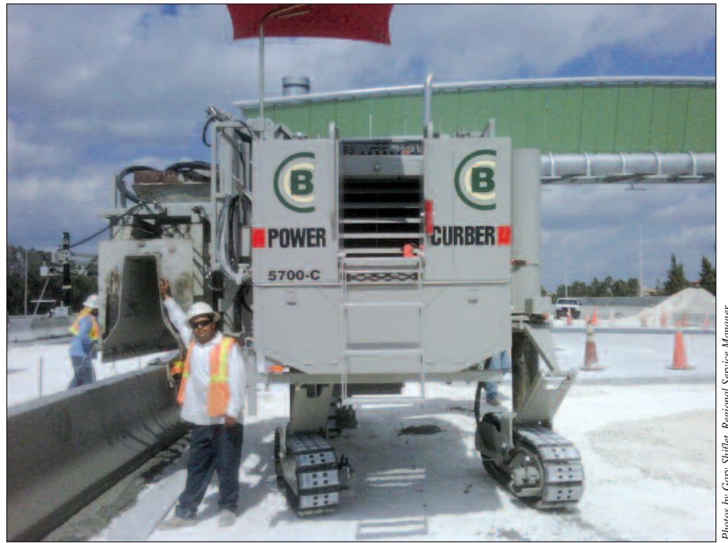
5700-C is shown with optional Barrier Mold Lift, Polyurethane Track Pads, and All Crawler Steering. The machine is on a barrier wall job in Miami, FL.
