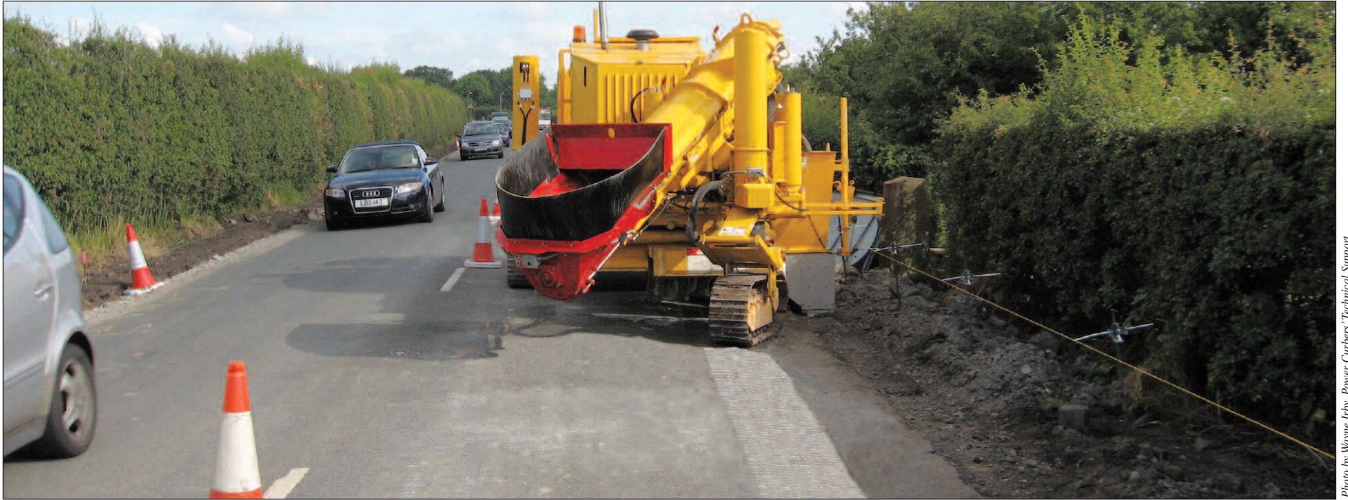
The compactness of the 5700-C and standard swivel chute make it possible to pour in a single 10-foot lane (3m)
