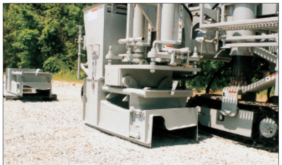
The machine with Quick-Connect Option does most of the work when it's time to change the mold
